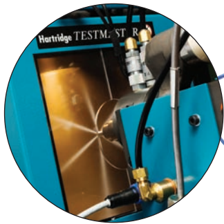
Figure 1 HH705 Spray pattern testing
